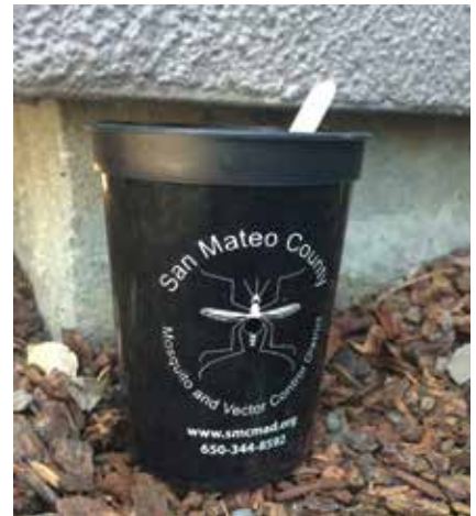
Aedes traps are simple in design — a dark container with a bit of water encourages females to lay their eggs on a paper in the container. Staff retrieve the papers and inspect for eggs.
