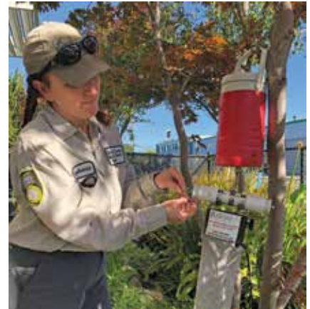
Vector Control Technician Stephanie sets a carbon-dioxide baited trap to capture adult mosquitoes to test for West Nile virus.
