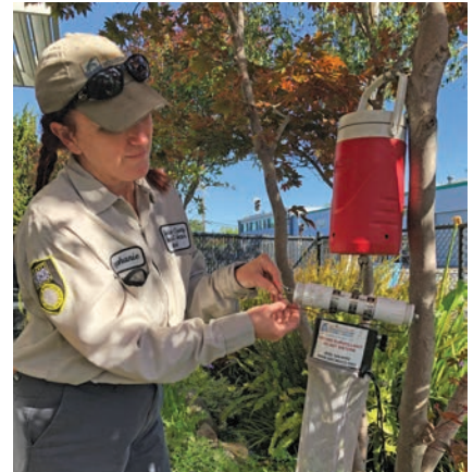
Vector Control Technician Stephanie sets a carbon-dioxide baited trap to capture adult mosquitoes to test for WNV.
